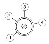
operational. Warning lights illuminated. Key position when driving. 4. Start — cranks the engine. Release the key as soon as the engine starts.
